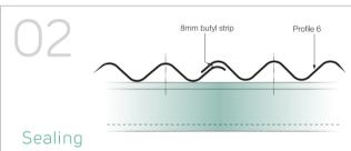
Lap sealant to be 8mm diameter butyl strip sealant, positioned as shown. Gun grade sealants are not suitable. When end laps are double sealed, the second strip of sealant should be 100-200mm below the fasteners.
